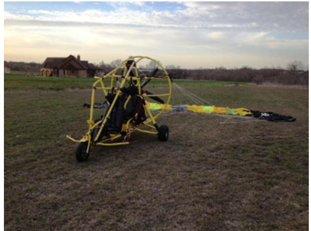
The Airwolf has undergone a complete preflight and the canopy is laid out behind the cart inverted and stacked. (John Craparo)
