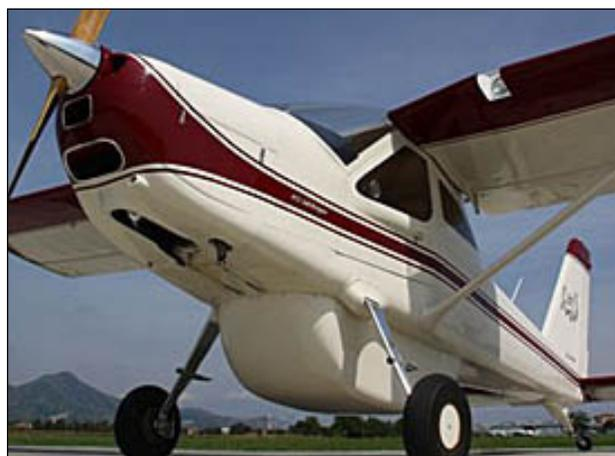
The cargo pod added to the ruggedness of a tail dragger should make Tecnam's new model appeal to bush flying enthusiasts.
