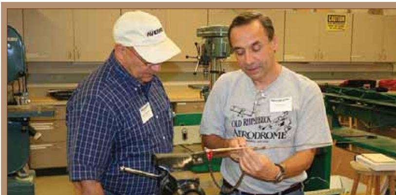
Gabe Dellaventura and John team up to properly tension an aileron control wire during the first week of class. (photo Jason Golden)
