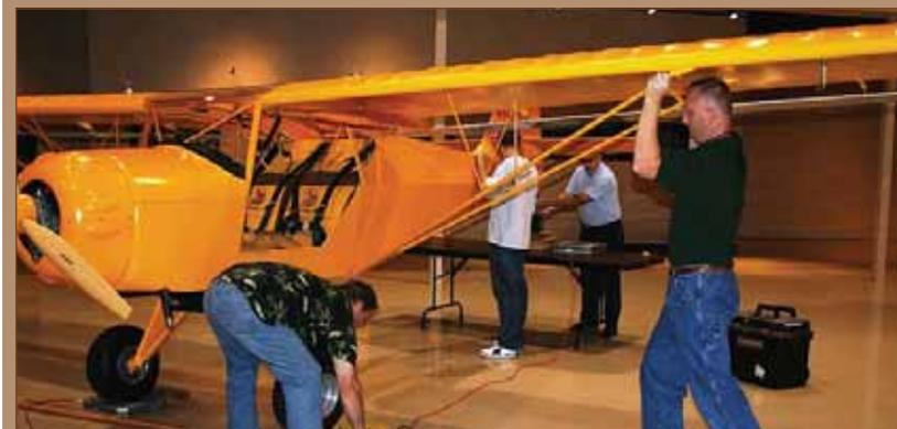
One team works to get an accurate revised weight & balance on a Kit Fox as they lift a wing so a scale can be placed under the main landing gear. (photo John Craparo)
